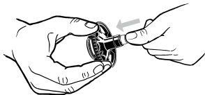
Push the cap cylinder out of the cap housing
