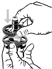
Screw on Filling Chamber Cap
